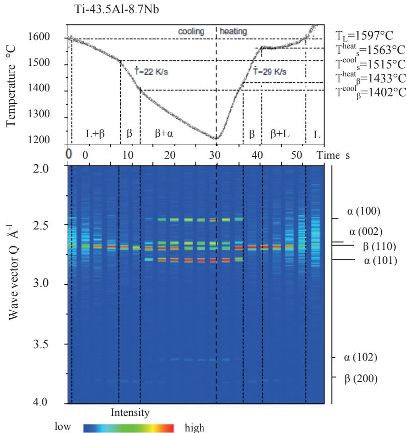
Figure 9: Time evolution of the temperature and the X-ray diffraction spectra during a solidification cycle of the Ti-43.5Al-8.7Nb alloy. The temperature–time profiles (top) are synchronised with the spectra (bottom) for the typical cooling and heating stages of the solidification cycle. The brightness in the intensity maps corresponds to the diffracted radiation intensity. The Bragg peaks of the crystalline phases are assigned at the right-hand side [56].
