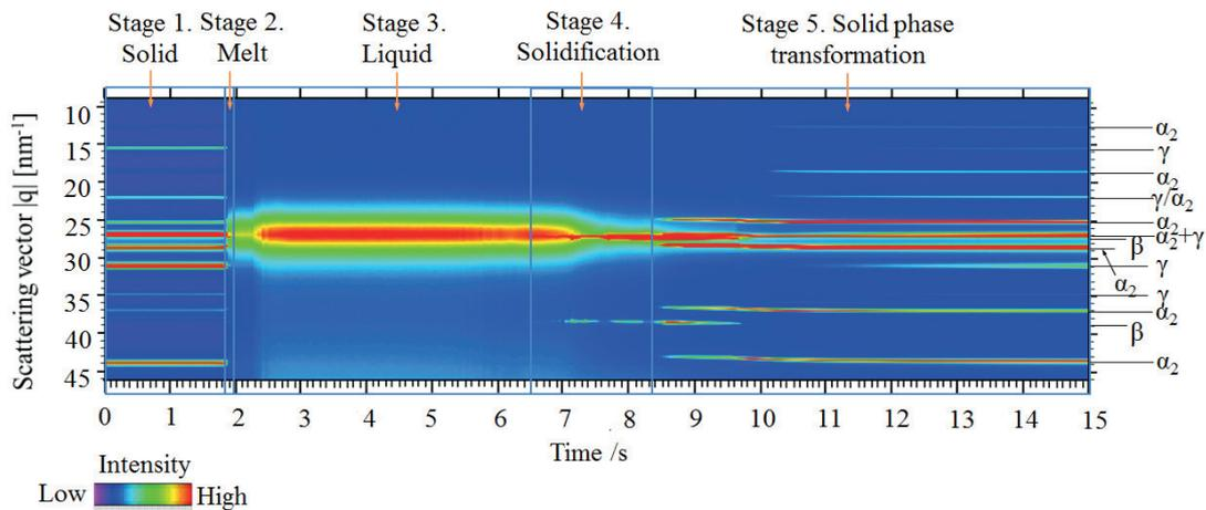
Figure 50: An example of time-resolved X-ray diffraction signals observed during the melting and solidification of TNB-V5 material.
