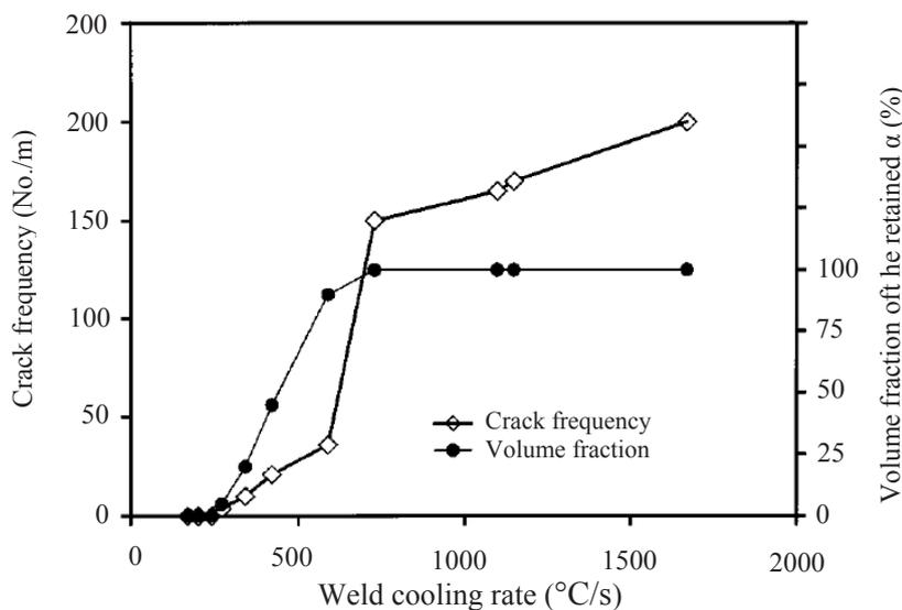
Figure 10: The weld crack frequency and the volume fraction of the retained  $\alpha$  phase in the weld vs. the calculated cooling rate [58].
