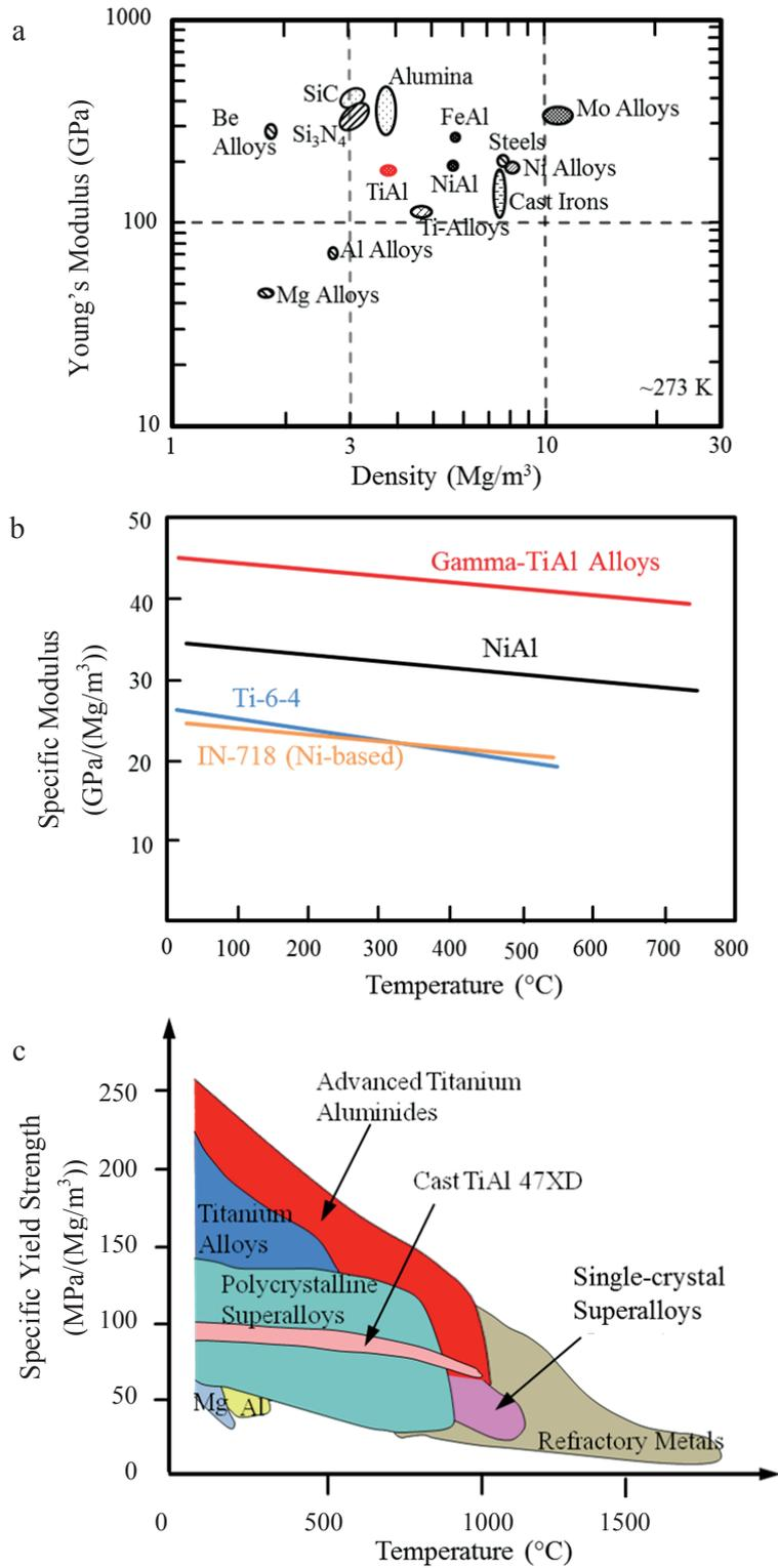
Figure 1: (a) Densities and Young's moduli of various structural materials. Certain density-normalised specific properties of structural alloys and selected intermetallics are also presented: (b) specific modulus versus temperature and (c) specific strength versus temperature [1, 3].
