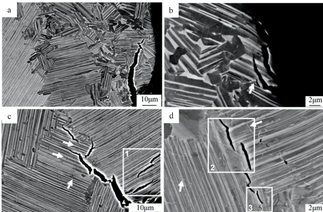
Figure 34: SEM observations in BSE mode of the microstructure of a heat-treated specimen after tensile testing at the fracture tip: (a) macroscopic view, (b) translamellar microcracking, (c) interlamellar microcracking, and (d) delamination separation through the  $\alpha_2$  phase and interlamellar debonding. The tensile loading was in the horizontal direction.
