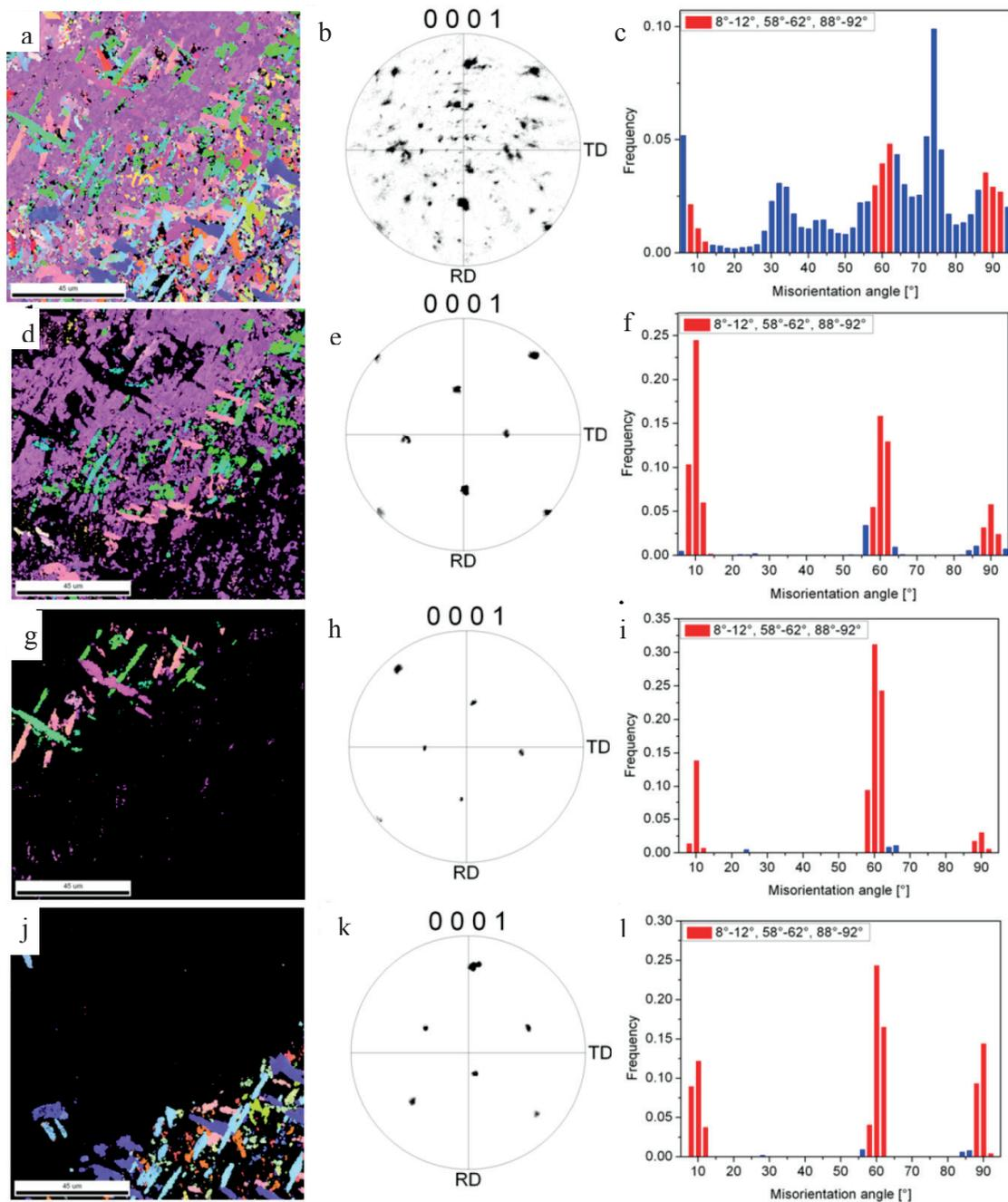
Figure 41: EBSD measurements of the  $Ti_3Al$  phase of the welding zone: (a) a texture map of all  $\alpha_2$  phase, (b) a pole figure of all  $\alpha_2$  phase (c) the misorientation angles between neighbouring grains; (d), (g) and (j) texture maps of three groups of  $\alpha_2$  grains; (e), (h) and (k) the corresponding pole figures of the three grain groups; and (f), (i) and (l) the misorientation angles between neighbouring  $\alpha_2$  grains of three grain groups.
