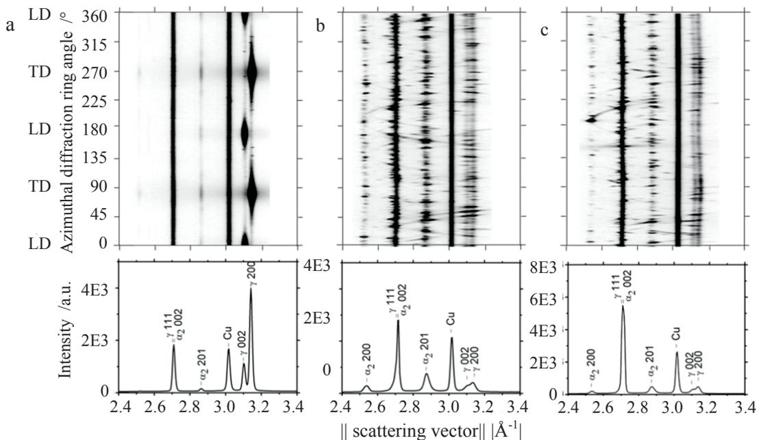
Figure 35: X-ray diffraction morphologies of the as-welded specimen: (a) base material, (b) welding zone, and (c) near-heat affected zone. The Debye-Scherrer diffraction rings have been unrolled into lines and azimuthally integrated. LD/TD denotes the longitudinal/transversal direction of the weld.
