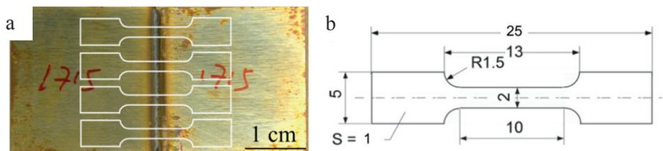
Figure 23: (a) A sketch illustrating the extraction of a tensile specimen from the middle of a weld. (b) Geometry of the micro tensile specimen. The unit is mm.
