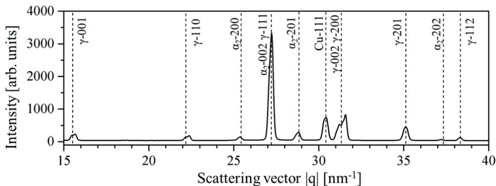
Figure 46: X-ray diffraction patterns (azimuthally averaged scattering intensity versus scattering vector  $|q|$ ) of the base material.
