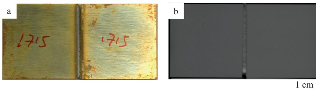
Figure 26: (a) Example of a specimen welded in the furnace. (b) Radiography of the specimen.
