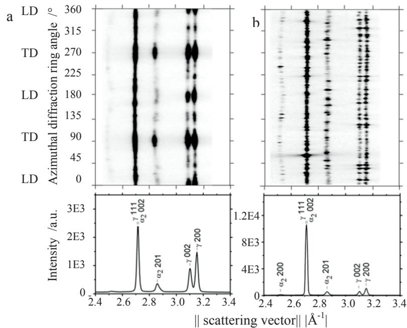
Figure 37: X-ray diffraction morphologies of the heat-treated specimen after tensile deformation at 750°C with an initial strain rate of  $1.67 \times 10^{-5} \text{ s}^{-1}$ : (a) base material and (b) welding zone (the specimen fractured at the welding zone). The diffraction morphologies were treated in the same manner as in Figure 35.
