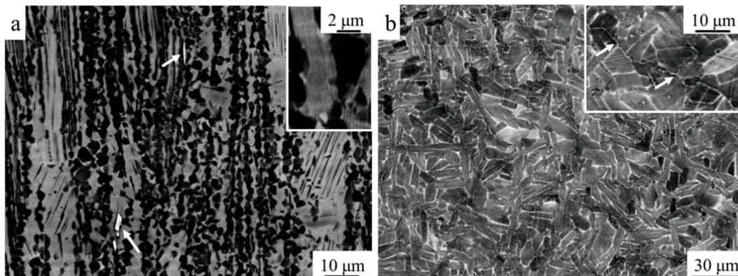
Figure 49: (a) Microstructure of the extruded rod (the extrusion direction is vertical). The arrows indicate borides parallel to the extrusion direction. The inset shows the details of the lamellae. (b) Microstructure of the melt zone after solidification, after laser melting of 300 W for 1.8 s. The arrows indicate the borides.
