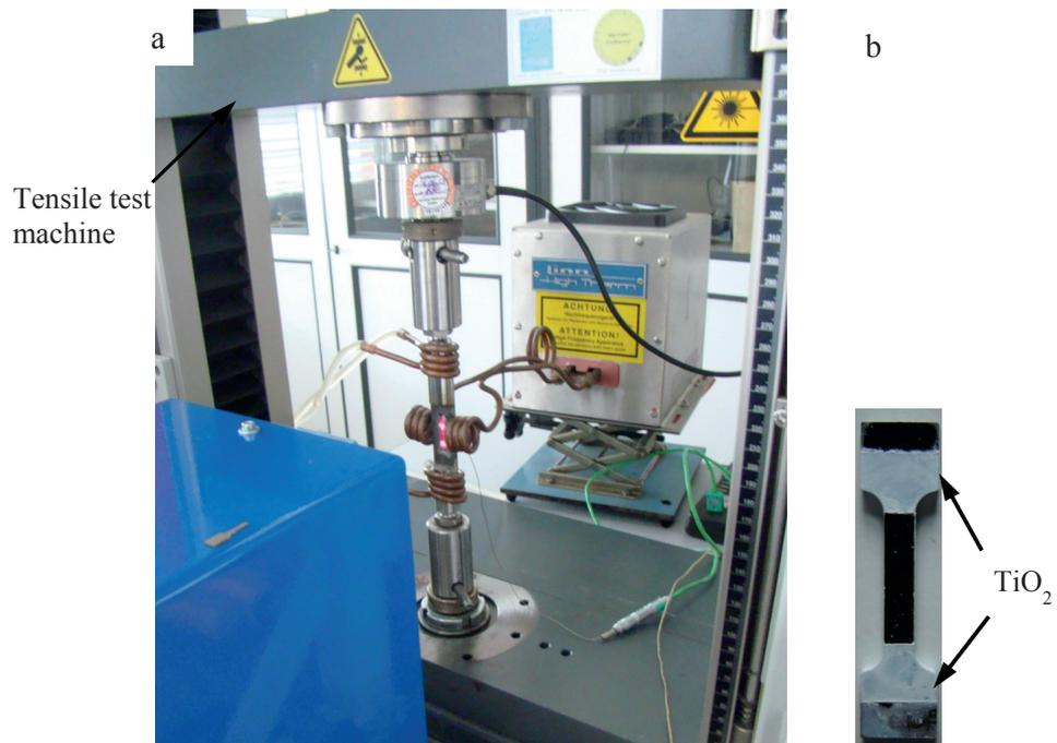
Figure 24: (a) Equipment for tensile tests and (b) a micro-tensile specimen. The length between the TiO<sub>2</sub> segments was measured using a laser extensometer during tensile testing.
