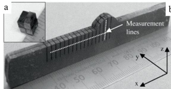
Figure 14: Specimens — (a) a set of cuboids and (b) a comb — used to determine the “stress-free” parameter  $d_0$  [82].
