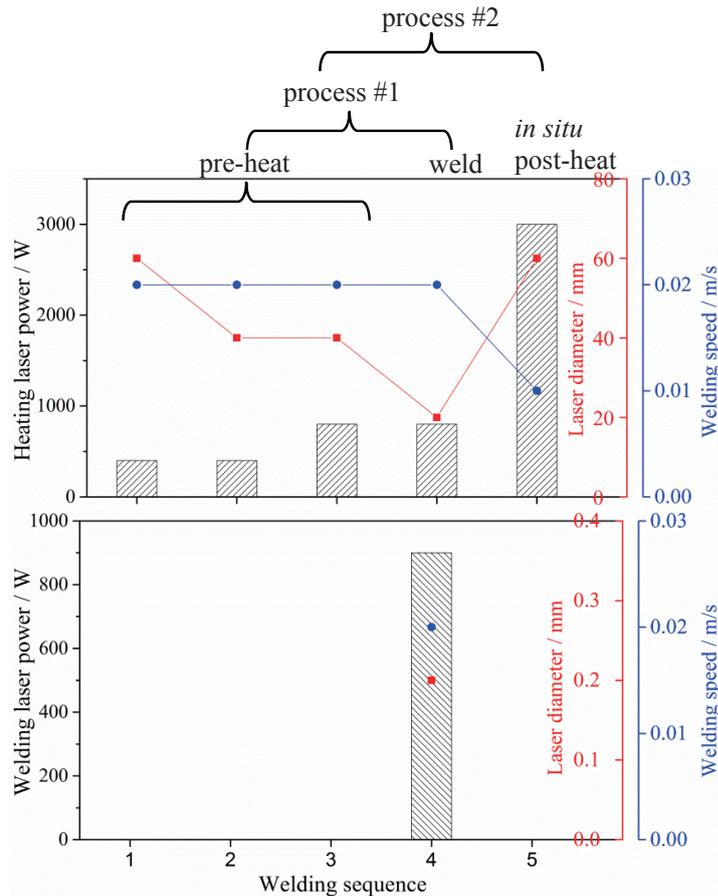
Figure 44: Dual-laser-beam welding parameters. Sequence 1-3: preheating with defocused laser. Sequence 4: welding and heating. The defocused laser is 2 mm behind the welding laser. Sequence 5: in situ post heating. The bars shows the energy input, the red dots indicating the laser diameter and the blue dots demonstrate the welding speed.
