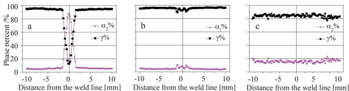
Figure 48: Phase percentages (volume percentages) of  $\gamma$  and  $\alpha_2$  across the welding zones of samples (a) 1, (b) 2, and (c) 3 as determined from the diffraction patterns.
