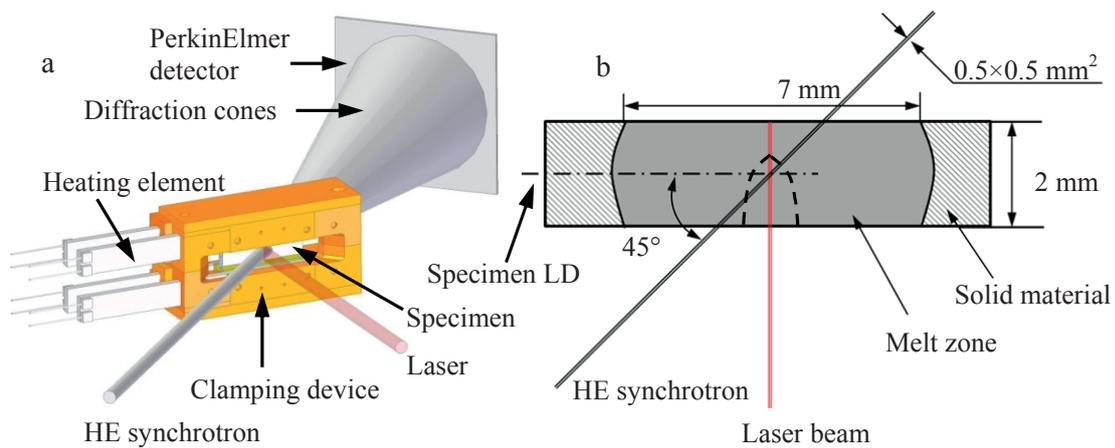
Figure 19: (a) Experimental set-up for the HEXRD *in situ* laser welding experiment. (b) Sketch of the geometry of the welding zone (top view) for phase transformation. Note that the melt zone of 7 mm in diameter developed during the late stage of the melting. The dashed line describes the shape of the melt zone in the initial stage.
