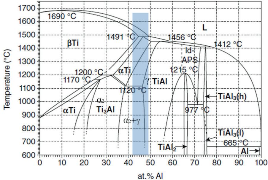
Figure 4: Binary Ti-Al phase diagram, according to the assessment of Schuster and Palm [35].
