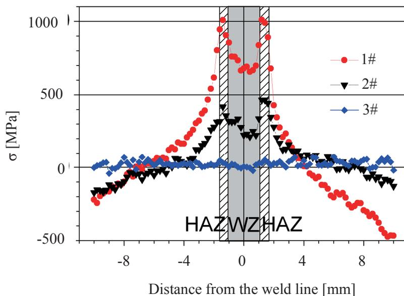
Figure 47: The longitudinal residual stresses of samples 1, 2, and 3, as determined via X-ray diffraction. The typical error is 30–50 MPa.
