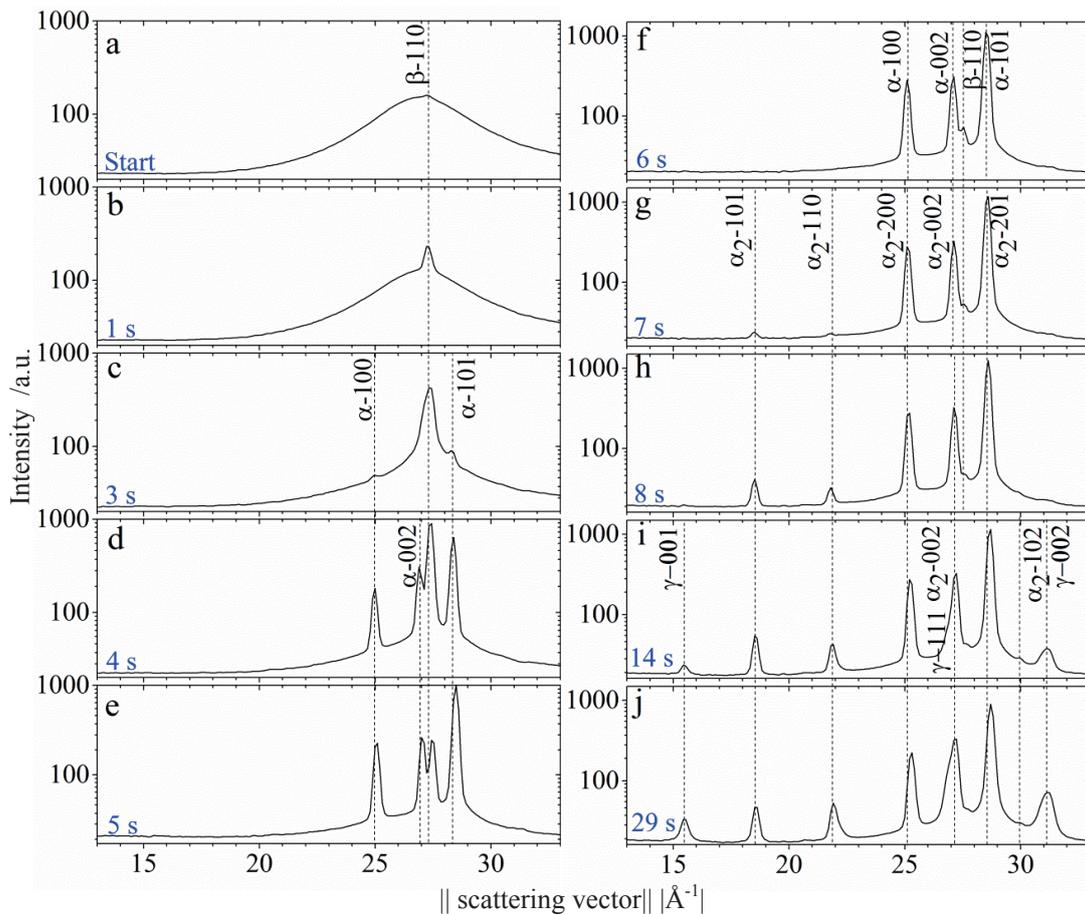
Figure 53: X-ray diffraction patterns observed during solidification, revealing the phase compositions (a) at the start of solidification and after (b) 1 s, (c) 3 s, (d) 4 s, (e) 5 s, (f) 6 s, (g) 7 s, (h) 8 s, (i) 14 s, and (j) 29 s. Heating temperature: 800 °C.
