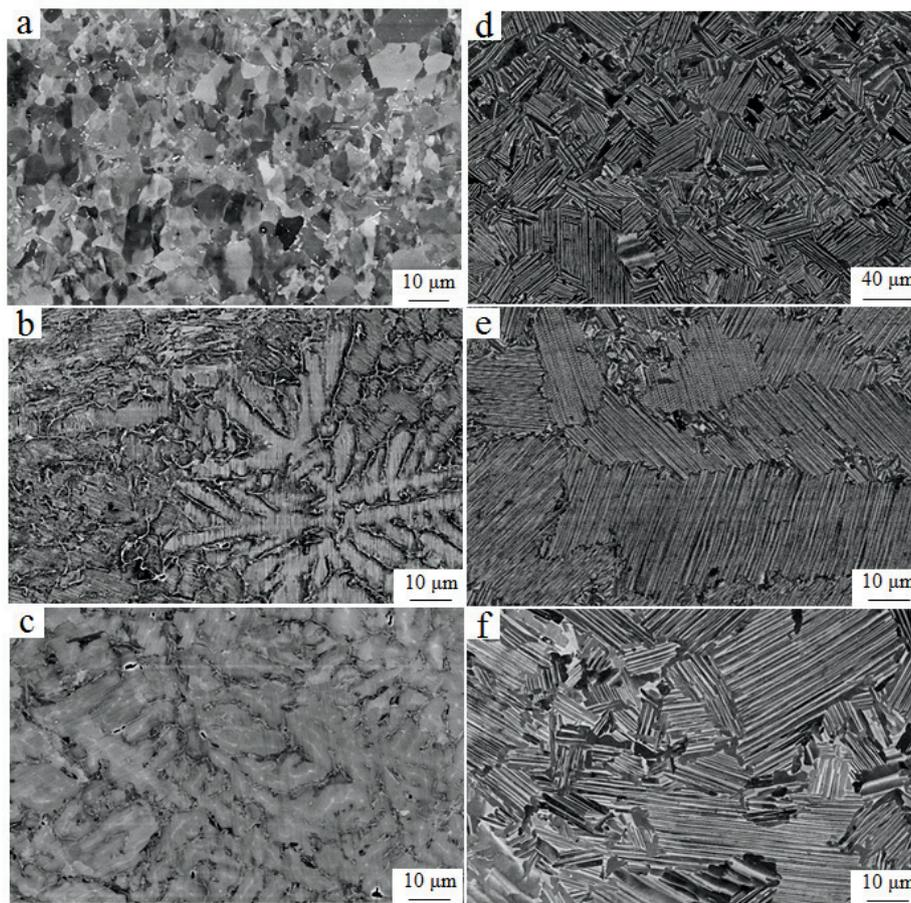
Figure 27: SEM observations of microstructures in BSE mode: (a), (b) and (c) are of the as-welded specimen, and (d), (e) and (f) are of the heat-treated specimen. (a), (d) base material; (b), (e) welding zone; and (c), (f) welding zone of the specimen after tensile testing.
