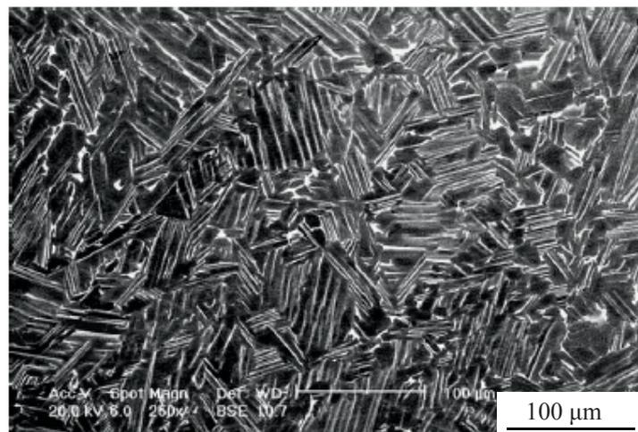
Figure 8: BSE micrograph of a sample of Ti-46Al-8Nb taken from a 20 mm diameter sample cut from an ingot, oil quenched to room temperature from 1360°C and aged at 1320°C for 2 h, exhibiting a typical convoluted microstructure [28].
