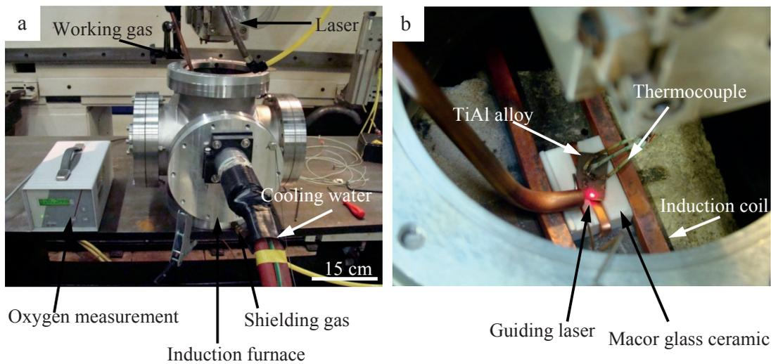
Figure 16: (a) Experimental set-up for induction-furnace heating and (b) welding details for thermocouple temperature measurements. Induction heating experiments were carried out in Fraunhofer Institute for laser technology.
