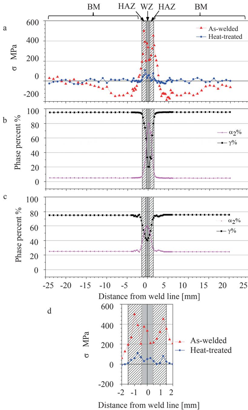
Figure 29: (a) Longitudinal stress maps along the welding lines of as-welded and heat-treated specimens. Phase distributions in the (b) as-welded and (c) heat-treated specimens. (d) The details of the residual-stress distributions in the welding zone and heat affected zone regions. BM: base material, HAZ: heat-affected zone, WZ: welding zone.
