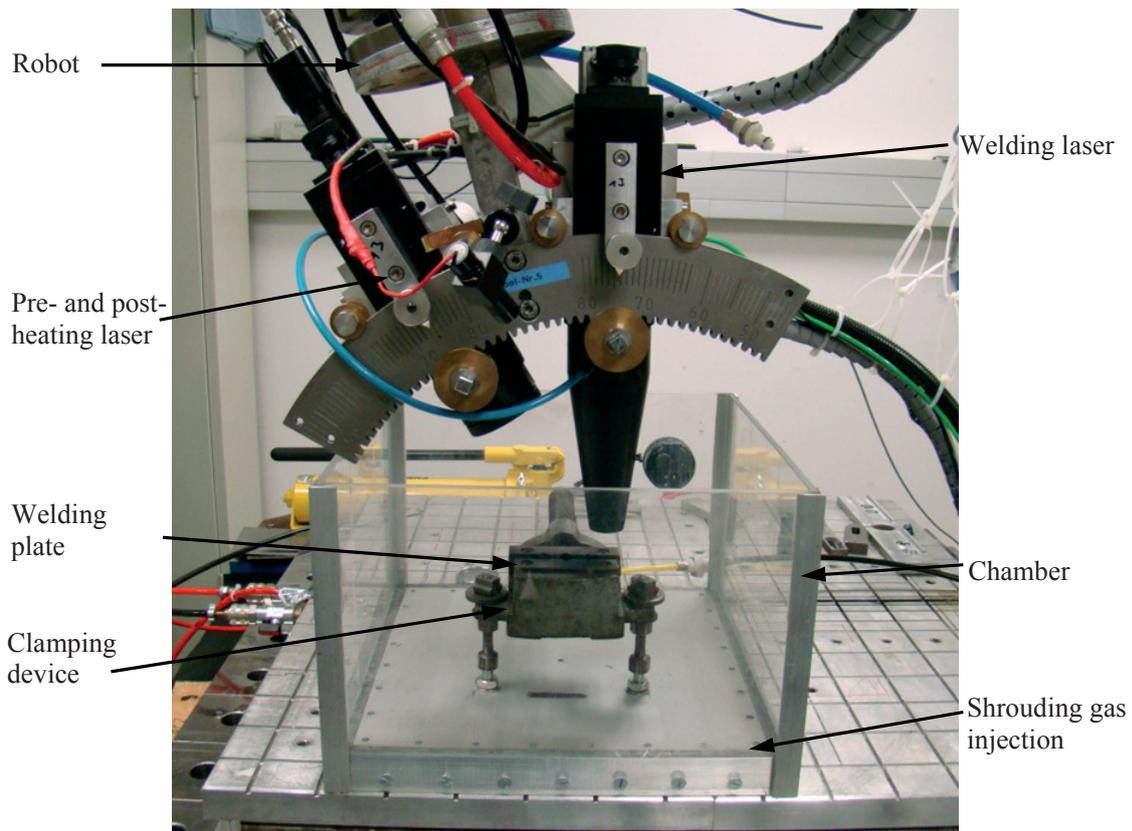
Figure 17: Dual-laser-beam welding set-up.
