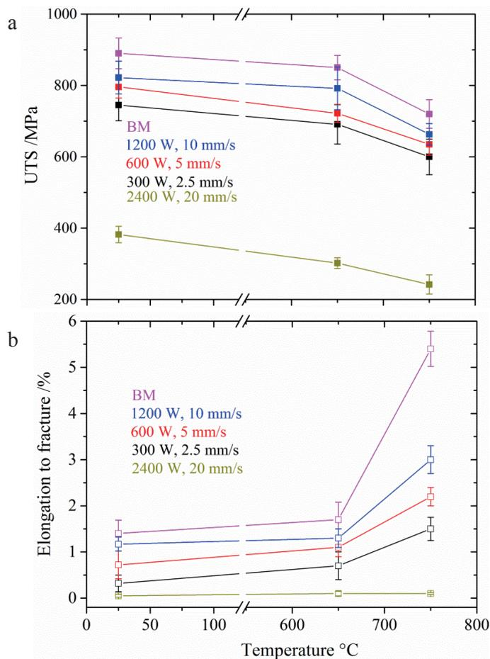
Figure 57: (a) UTS and (b) elongation-to-fracture values for bead-on-plate welded specimens prepared using four different sets of welding parameters at 25°C, 650°C and 750°C.
