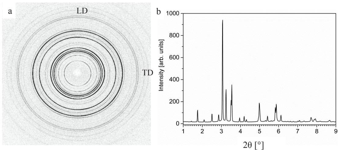
Figure 22: (a) An example showing the diffraction pattern of TNB-V5. (b) The pattern is integrated to obtain the azimuthally averaged scattering intensity as a function of the diffraction angle  $2\theta$ .
