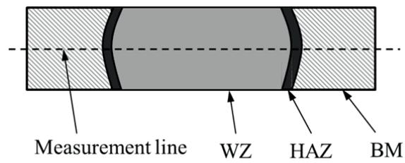
Figure 25: Micro hardness measurement position.
