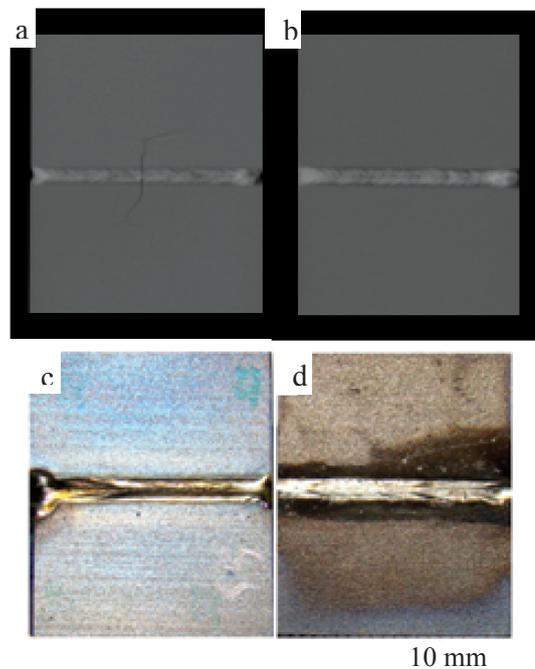
Figure 38: (a) Representative radiograph of specimen #1. (b) Radiograph of crack-free specimen #3. (c) Top and (d) bottom sides of specimen #3.
