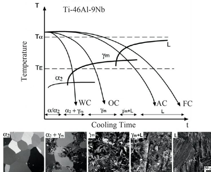
Figure 7: Schematic CCT diagram of a high-Nb-bearing  $\gamma$ -TiAl-based alloy, showing the microstructures that form as a result of different cooling rates [44].  $\gamma_m$ : massive  $\gamma$ . L: lamellae. WC: water cooling. OC: oil cooling. AC: air cooling. FC: furnace cooling.
