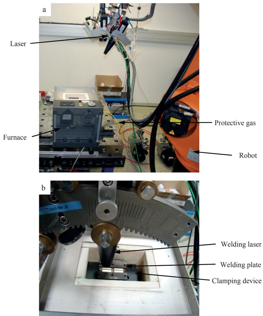
Figure 15: (a) Experimental set-up for furnace heating and welding and (b) a detail view of the welding with a focused laser perpendicular to the specimen surface.
