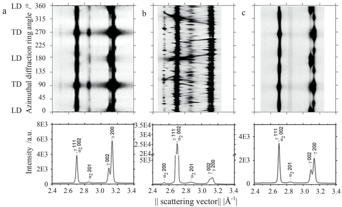
Figure 36: X-ray diffraction morphologies of the as-welded specimen after tensile testing at 750°C with an initial strain rate of  $1.67 \times 10^{-5} \text{ s}^{-1}$ : (a) base material, (b) welding zone and (c) fracture tip (the specimen fractured at the base material). The diffraction morphologies were treated in the same manner as in Figure 35.
