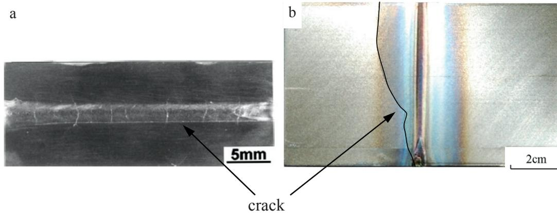
Figure 2: (a) Transverse cracking in a weld at a cooling rate of  $1670^{\circ}\text{C/s}$  [11]. (b) A longitudinal crack.
