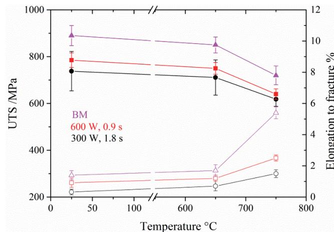
Figure 56: UTS (solid symbols) and elongation-to-fracture (hollow symbols) values for base material and spot welded specimens prepared using two sets of welding parameters at 25°C, 650°C and 750°C.
