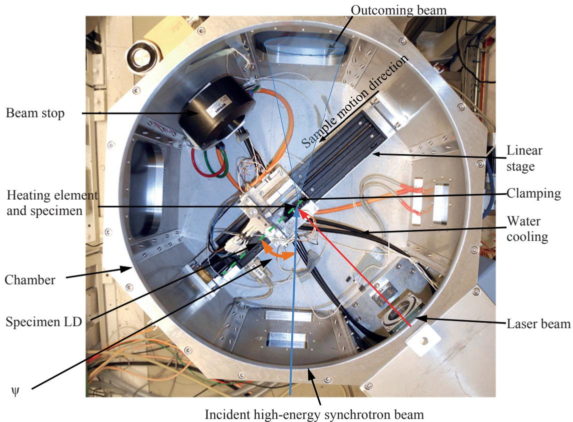
Figure 18: FLEXILAS welding chamber, top view (the symbol  $\psi$  represents the angle between the synchrotron beam and the specimen LD).
