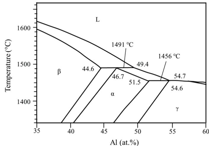
Figure 5: Section of the phase diagram calculated by Witusiewicz et al. for the peritectic reaction [34].
