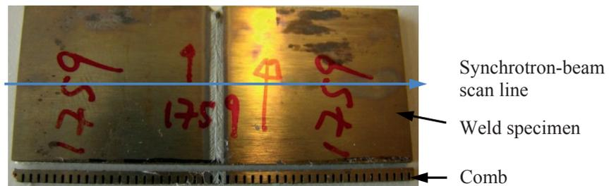
Figure 21: Electro-discharge machined comb used as a stress-free reference.
