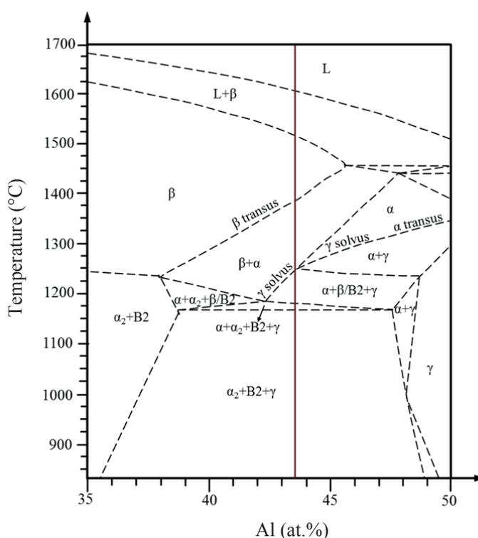
Figure 12: Experimental phase diagram of the alloy Ti-xAl-4Nb-1Mo-0.1B [23].
