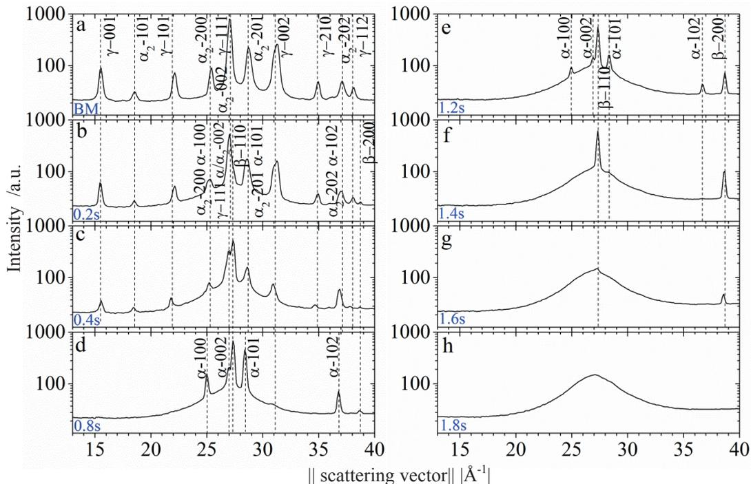
Figure 52: X-ray diffraction patterns observed during melting at a new position, revealing the phase compositions (a) of the base material and (b-h) at various times after the initiation of the laser melting process: (b) 0.2 s, (c) 0.4 s, (d) 0.8 s, (e) 1.2 s, (f) 1.4 s, (g) 1.6 s, and (h) 1.8 s. Laser power: 300 W.
