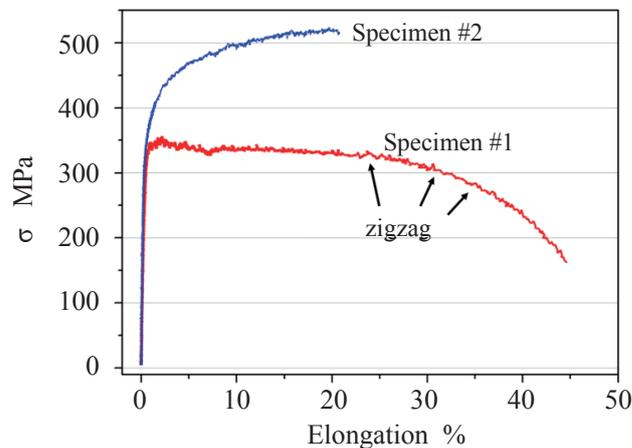
Figure 31: Tensile stress vs. elongation for as-welded (#1) and heat-treated (#2) specimens. The weld lines were oriented normal to the loading direction. The tensile tests were conducted at 750°C.
