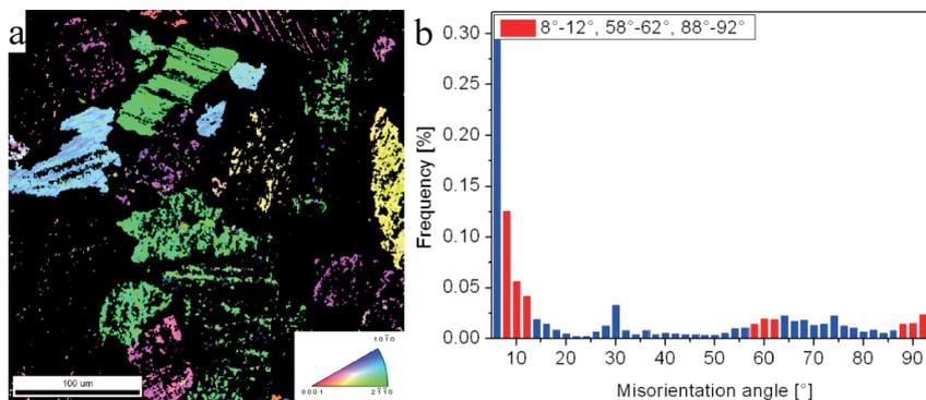
Figure 40: EBSD measurements of the  $Ti_3Al$  phase of the base material: (a) the texture map and (b) the misorientation angles between neighbouring  $Ti_3Al$  grains.
