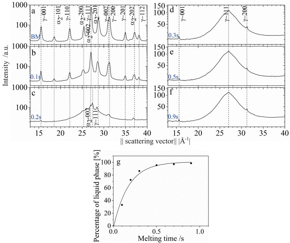
Figure 51: (a-f) X-ray diffraction patterns (azimuthally averaged scattering intensity versus scattering vector  $|q|$ ) acquired during the laser melting of TNB-V5, revealing the phase compositions (a) of the base material and (b-f) at various times after the initiation of the laser melting process: (b) 0.1 s, (c) 0.2 s, (d) 0.3 s, (e) 0.5 s, and (f) 0.9 s. (g) Volume fraction of the liquid phase during laser melting. Laser power: 600 W.
