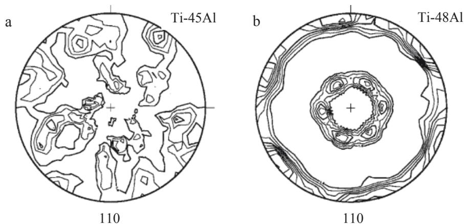
Figure 6: Pole figures of the  $\gamma$  (TiAl) phase determined from binary arc-melted buttons using neutron diffraction [39]: (a) Ti-45Al,  $\{110\}$  pole figure, maximum pole density 1.66 random; (b) Ti-48Al,  $\{110\}$  pole figure, maximum pole density 2.67 random.
