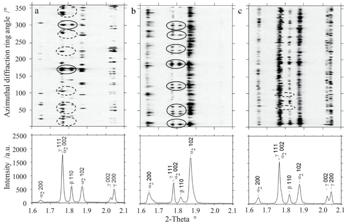
Figure 43: X-ray diffraction patterns of the (a) base material, (b) welding zone, and (c) annealed welding zone. The Debye-Scherrer diffraction rings have been unrolled into lines and azimuthally integrated. The solid and dashed ellipses indicate reflection pairs that correspond and do not correspond to the Burgers orientation relationship, respectively.
