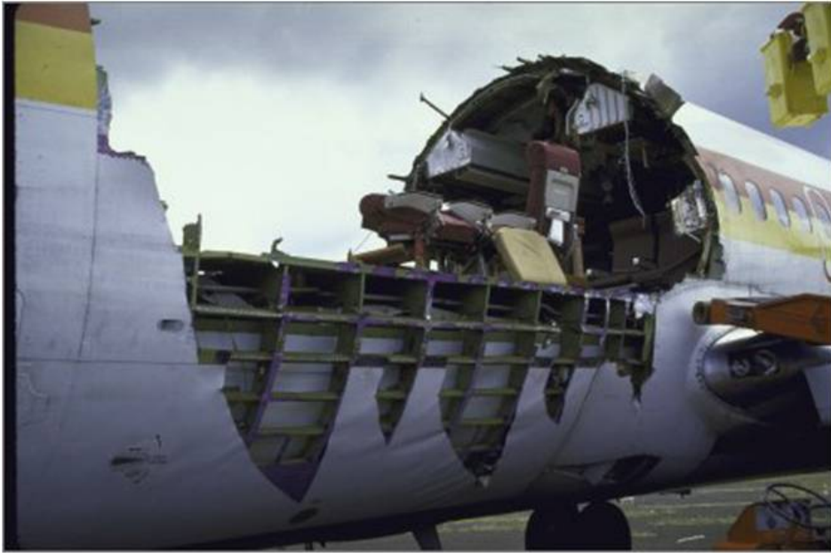
Figure 3.1: The severely damaged fuselage of the Aloha Airlines Boeing 737 (Learnmount, 2008), following the accident on April 28, 1988
