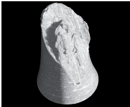
(a) 10 mm notch (Slant fracture)
