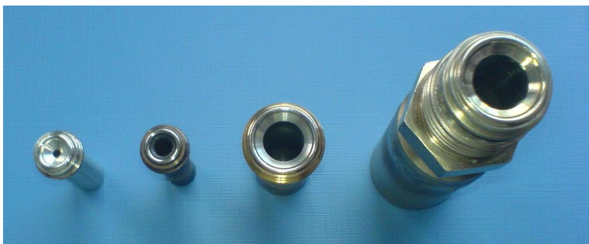
Figure 2.1: Cells of different inner diameter utilized for sorption measurements in the Sieverts' apparatus. Inner diameter from left to right: 2 mm, 4.5 mm, 10 mm and 15.2 mm.
