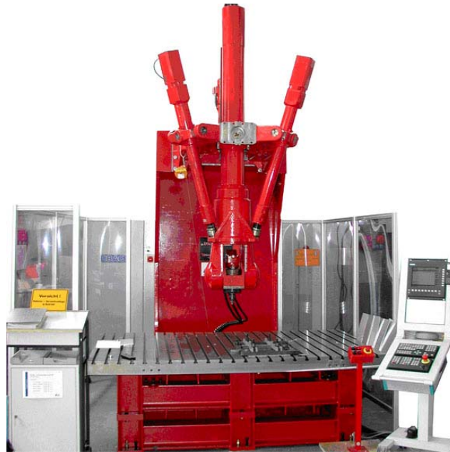
Figure 4-2 - Neos Tricept 805 Robot system used to produce the joints by FSW, with the ability to perform welds of up to 45kN axial load.
